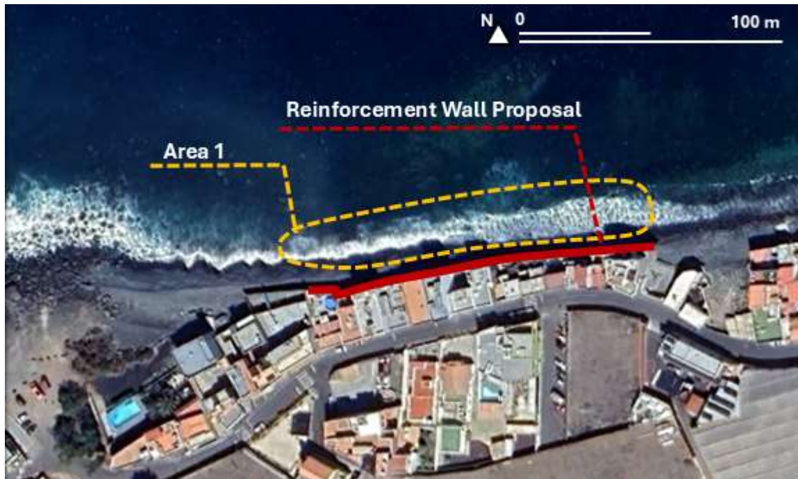
Figure 55. Proposed perimeter wall in Area 1
